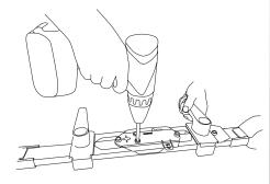
Drill bit (screw length = 16.3 mm): 3.6x9 mm
